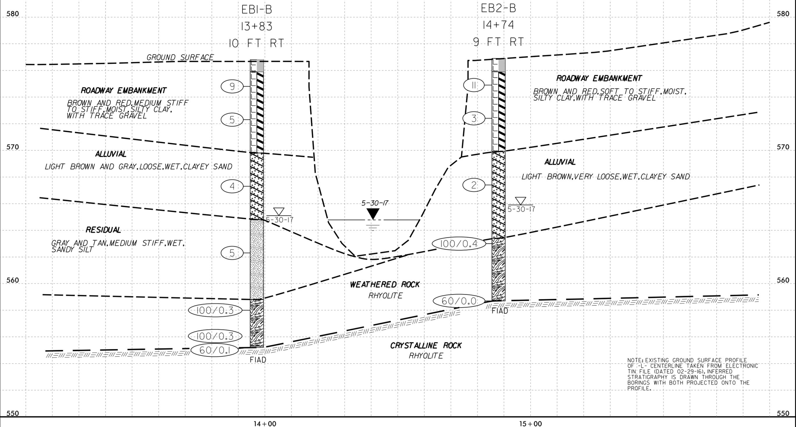
NOTE: EXISTING GROUND SURFACE PROFILE OF -L- CENTERLINE TAKEN FROM ELECTRONIC TIN FILE (DATED 02-29-16). INFERRED STRATIGRAPHY IS DRAWN THROUGH THE BORINGS WITH BOTH PROJECTED ONTO THE PROFILE.
