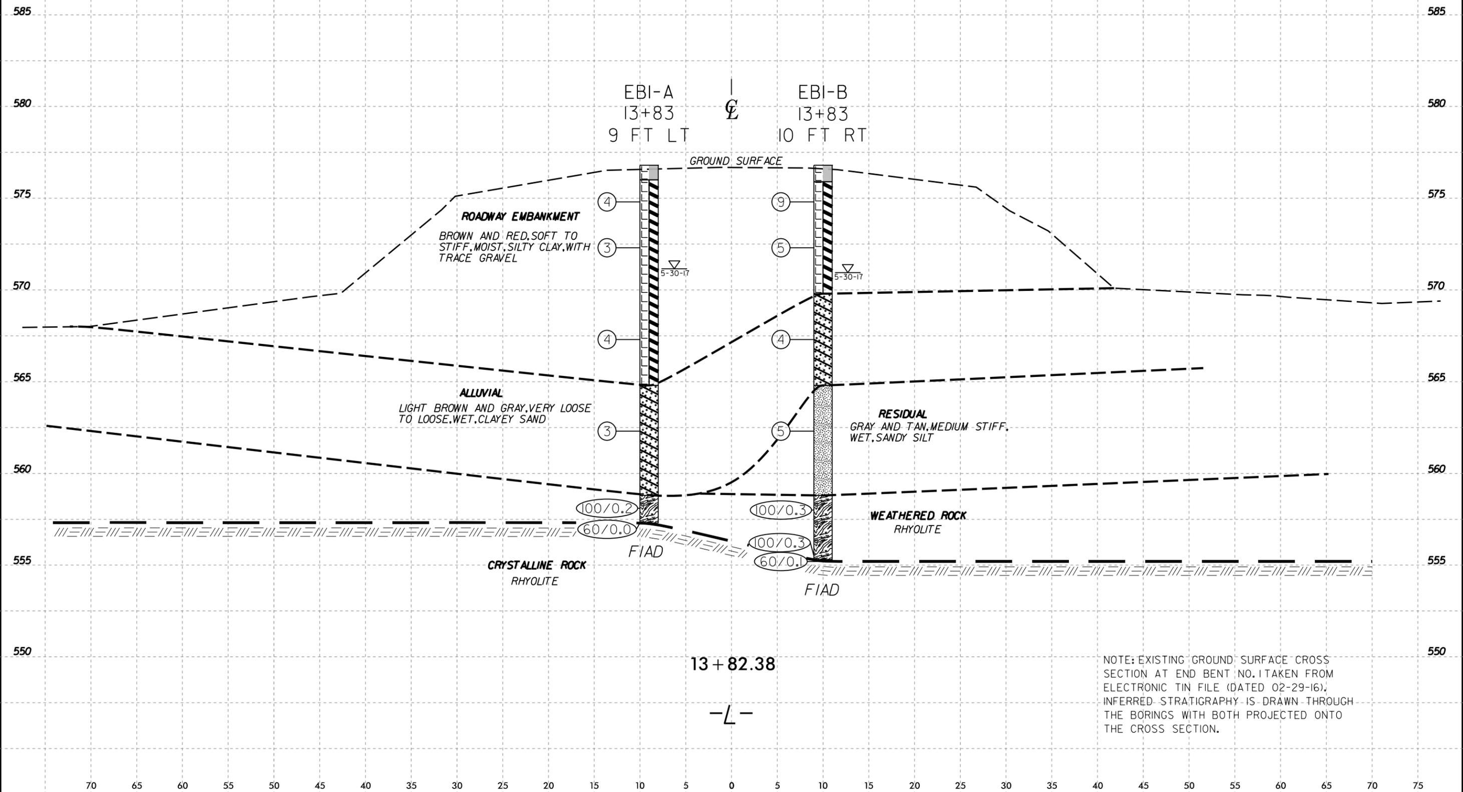
NOTE: EXISTING GROUND SURFACE CROSS SECTION AT END BENT NO. 1 TAKEN FROM ELECTRONIC TIN FILE (DATED 02-29-16), INFERRED STRATIGRAPHY IS DRAWN THROUGH THE BORINGS WITH BOTH PROJECTED ONTO THE CROSS SECTION.
